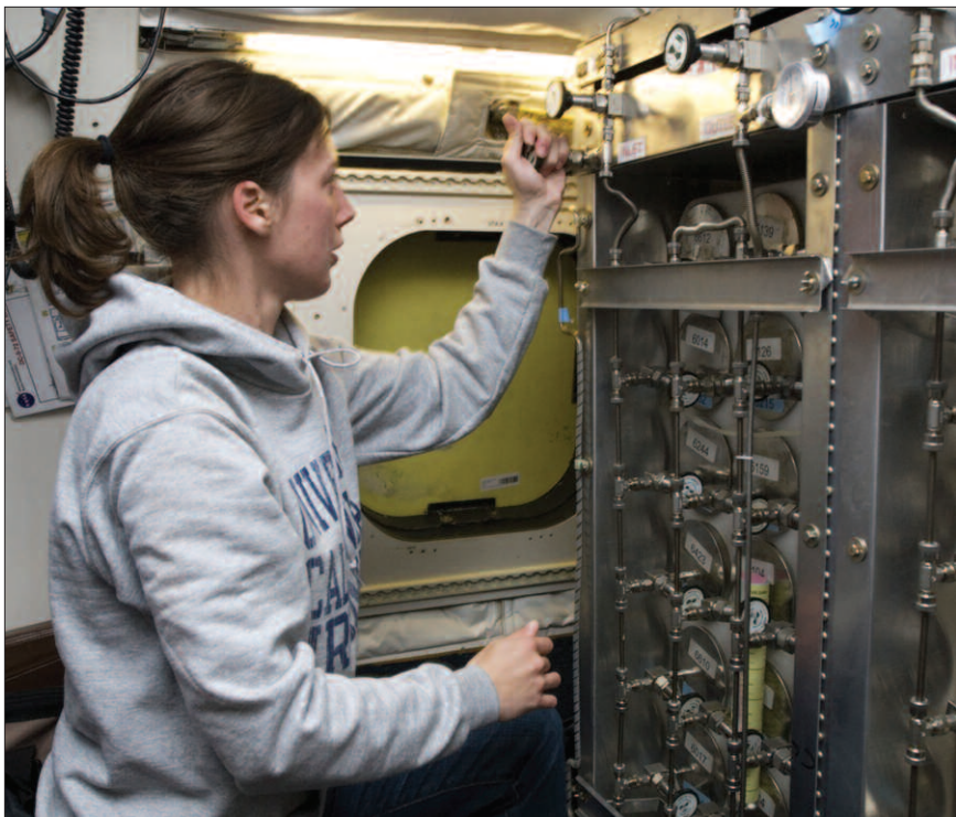
University of California, Irvine, graduate student Katrine Gorham operates an air sampler on a NASA DC-8 airplane during an Arctic Research of the Composition of the Troposphere from Aircraft and Satellites (ARCTAS) flight. (Courtesy NASA/Eric James)
