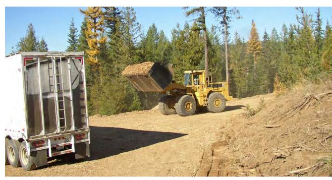
Forest debris is loaded into a chip van. The waste will be ground into a usable bio-product.
