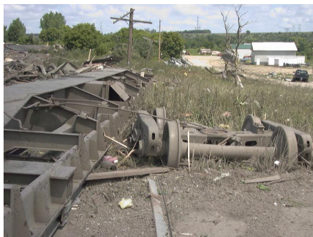
Figure 6: Damage to a flatbed railroad car from the Granite Falls, MN tornado, July 20, 2000. Notice the track runs along the upper left corner of the image, slightly uphill from the damage.
