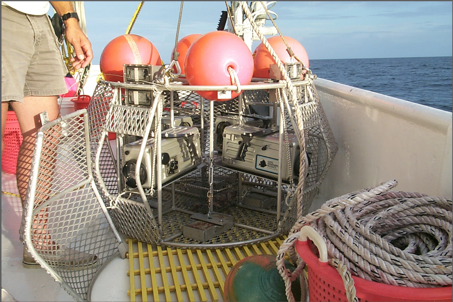
2001: Four camera pod using 4 Sony VX1000 digital camcorders in Gates housings with lasers.
