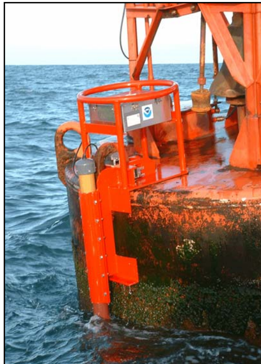
Figure 2. The prototype clamparatus deployed on Buoy 2C at the mouth of the Chesapeake Bay
