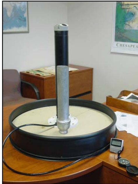
Figure 9. Calibration table with current profiler and steel pipe used to simulate the ATON's magnetic effect
