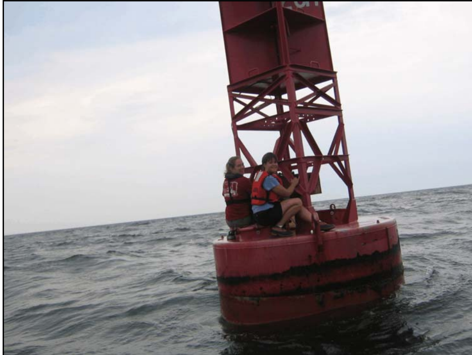
Figure 58. Calibrating the compass of the ATON current measurement system on LB 2CH
