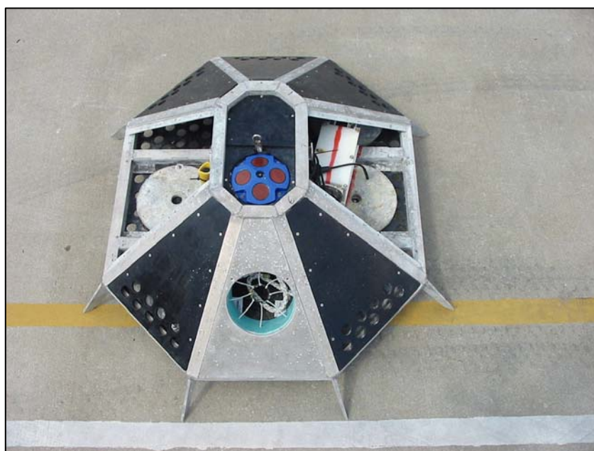
Figure 39. Seabed mooring with RDI ADCP
