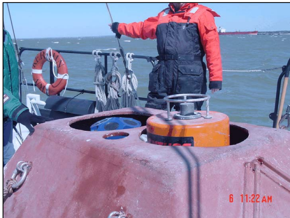
Figure 28. Bottom-mount for ADCP with pop-up buoy for recovery
