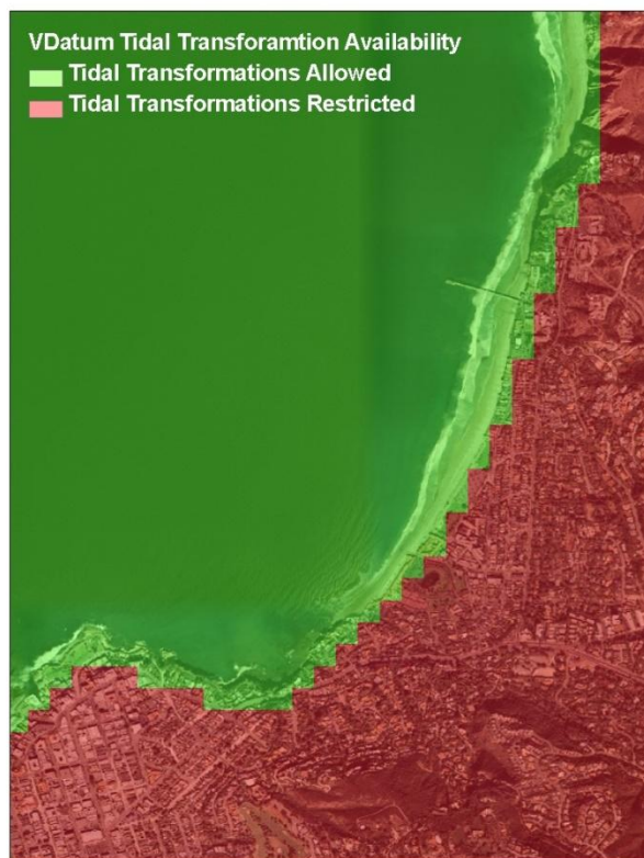
Figure 5.7. Illustrated are the areal extents of where VDatum allows/restricts tidal datum transformations.
