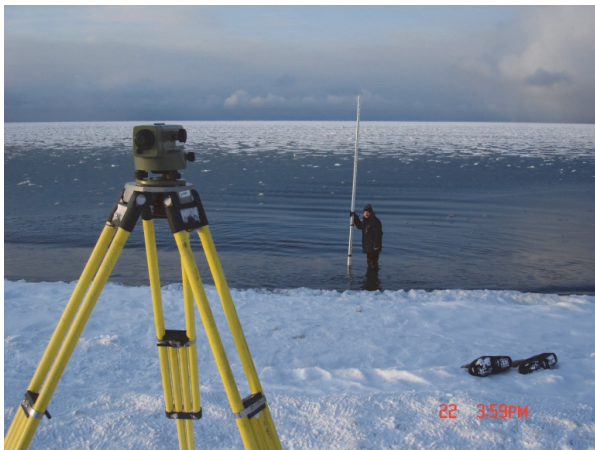
Figure 10a. "Staff shots" are a method of measuring the water level relative to the bench marks. October 2008.
