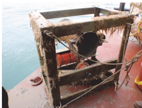
Figure 4b. Platform recovered after a 12 month long deployment
