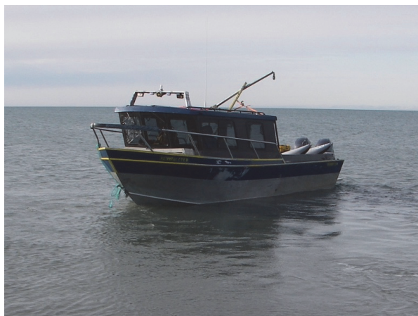
Figure 8a. Crawford Patkotak's boat with homemade davit used to deploy anchors in 2009, and recover anchors in 2010.
