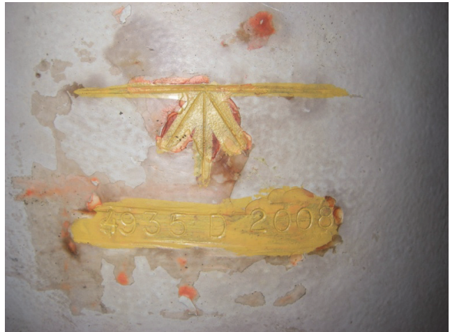
Figure 5b. Stamping and datum point for tidal bench mark 949 4935 D.
