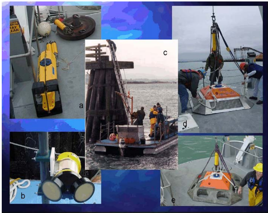
Figure 4. Equipment utilized during the 2002/2003 Humboldt Bay current survey consisted of (a) RDI WorkHorse ADCP in a subsurface buoy, (b) Sontek side looking profiler (SL-ADP), (c) mounted to the dolphin at Fairhaven Terminal, (d) bottom mounted ADCP housed in an aluminum base and (e) concrete base.
