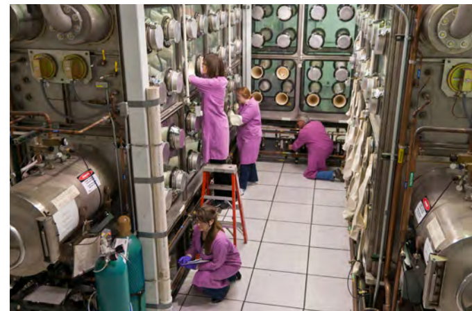
Researchers prepare gloveboxes for pyroprocessing tests.
