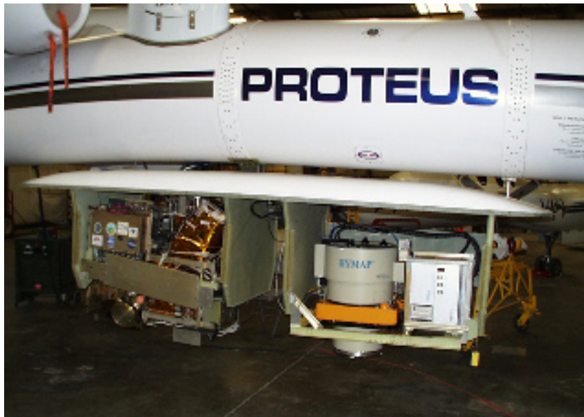
NASA Double Q-Bay Pod showing installation of NASA-JPL AVIRIS and Commercial HyMap Hyperspectral Remote Sensors.
