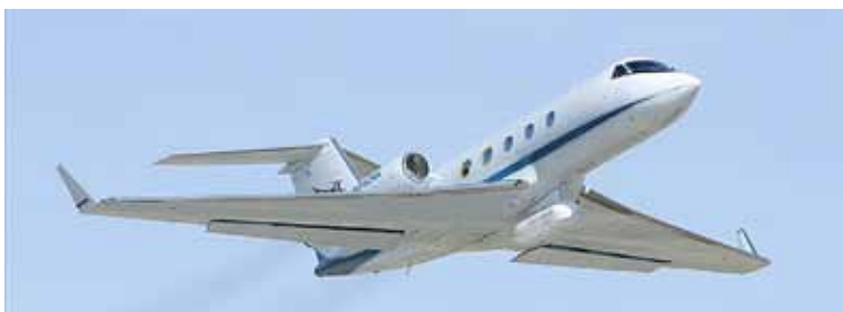
Figure 44. The JSC G-III Showing the UAVSAR Pod.
