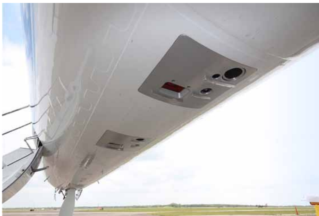
Figure 29. The MASS instrument was installed to make use of G-V nadir portals. Photo credit: NASA JSC
