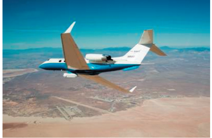
Figure 37: G-3 in flight over Edwards AFB with UAVSAR pod installed.
