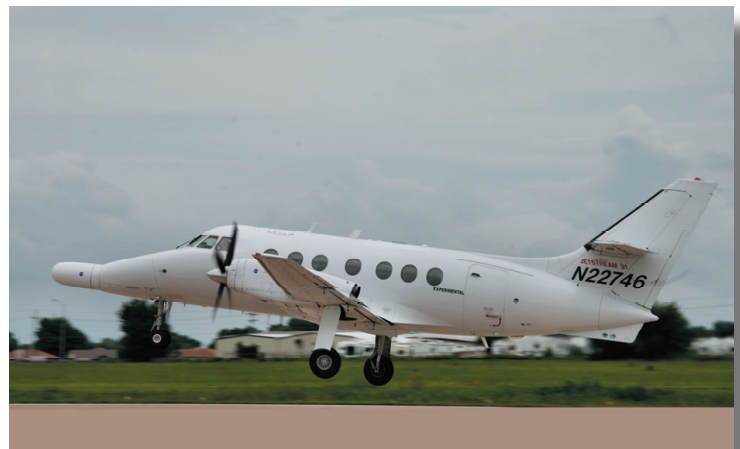
Figure 7: The J-31 landing at Ponca City Municipal Airport, Oklahoma. The CAR instrument is housed in the nose cone and views the earth and sky through a 190° aperture.
