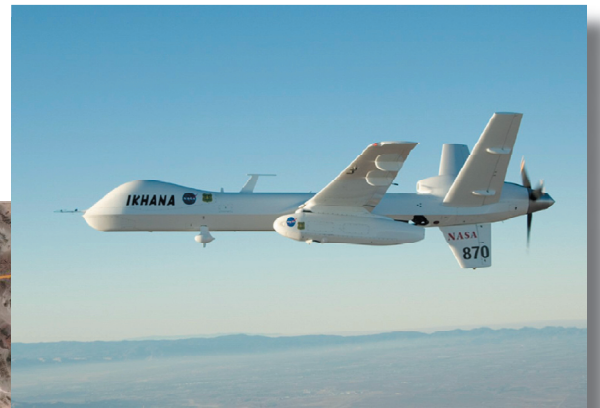
Fig. 19: Ikhana with AMS sensor in wing pod on its way to Southern California fires.
