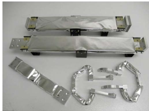
Figure 19: Proto-flight Heat Strap Segments
