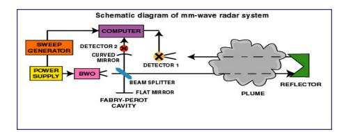
Argonne's system can determine both narrow and broad spectral features of airborne materials at pressures ranging from millitorr to atmospheric and at temperatures from ambient to 300°C. The ability to detect so many substances in such a wide range of conditions makes this mmW radar detection system useful for many types of applications.
