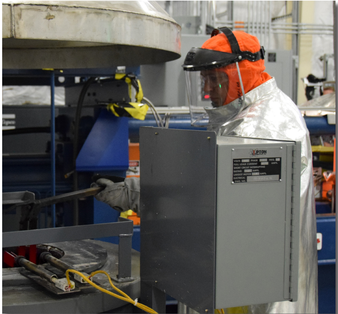
As part of a revived fuel fabrication technique, a technician removes a glowing billet of depleted uranium from a high temperature salt bath to place it into the extrusion press. Extrusion, rather than casting fuel, has the potential to be an easier and more efficient fuel fabrication process.
