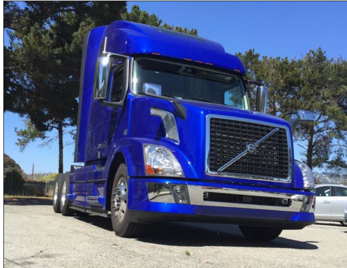
Figure 6. Photo. This truck, designed by Volvo, uses onboard sensors and vehicle-to-vehicle technology to form platoons with other equipped vehicles. (Source: Cambridge Systematics, Inc.)
