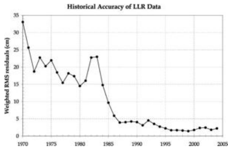
Figure 11. (Range Observation – Model) residuals showing the improvement in ground stations over the past four decades.
