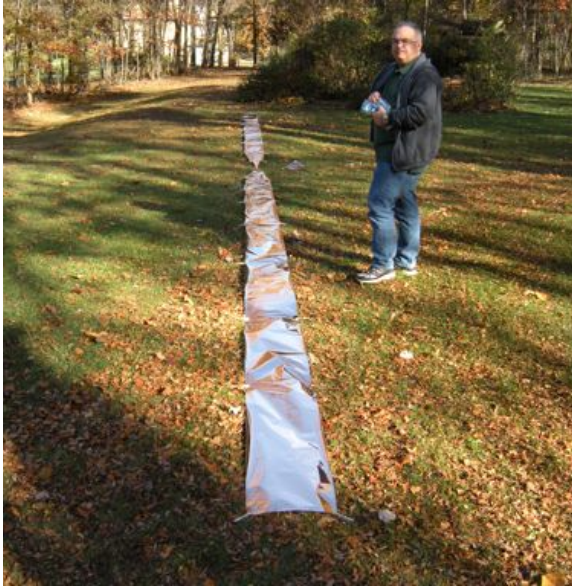
Figure 5. (Left) Polyimide film-based dipole antenna capable of being transported in a roll and deployed by unrolling on the lunar surface, being developed by NRL, NASA/GSFC, and JPL. (Right) Magnetic helix antenna capable of being constructed from memory metals and self deployed on the lunar surface, being developed by the NRAO. The antenna is wrapped around a support structure, which is required because of the high terrestrial gravity, but the antenna itself is not visible.
