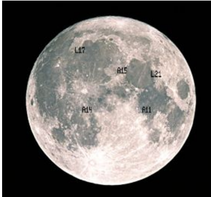
Figure 9. Placement of three Apollo LLR and the two Soviet LLR (L1 & L2).
