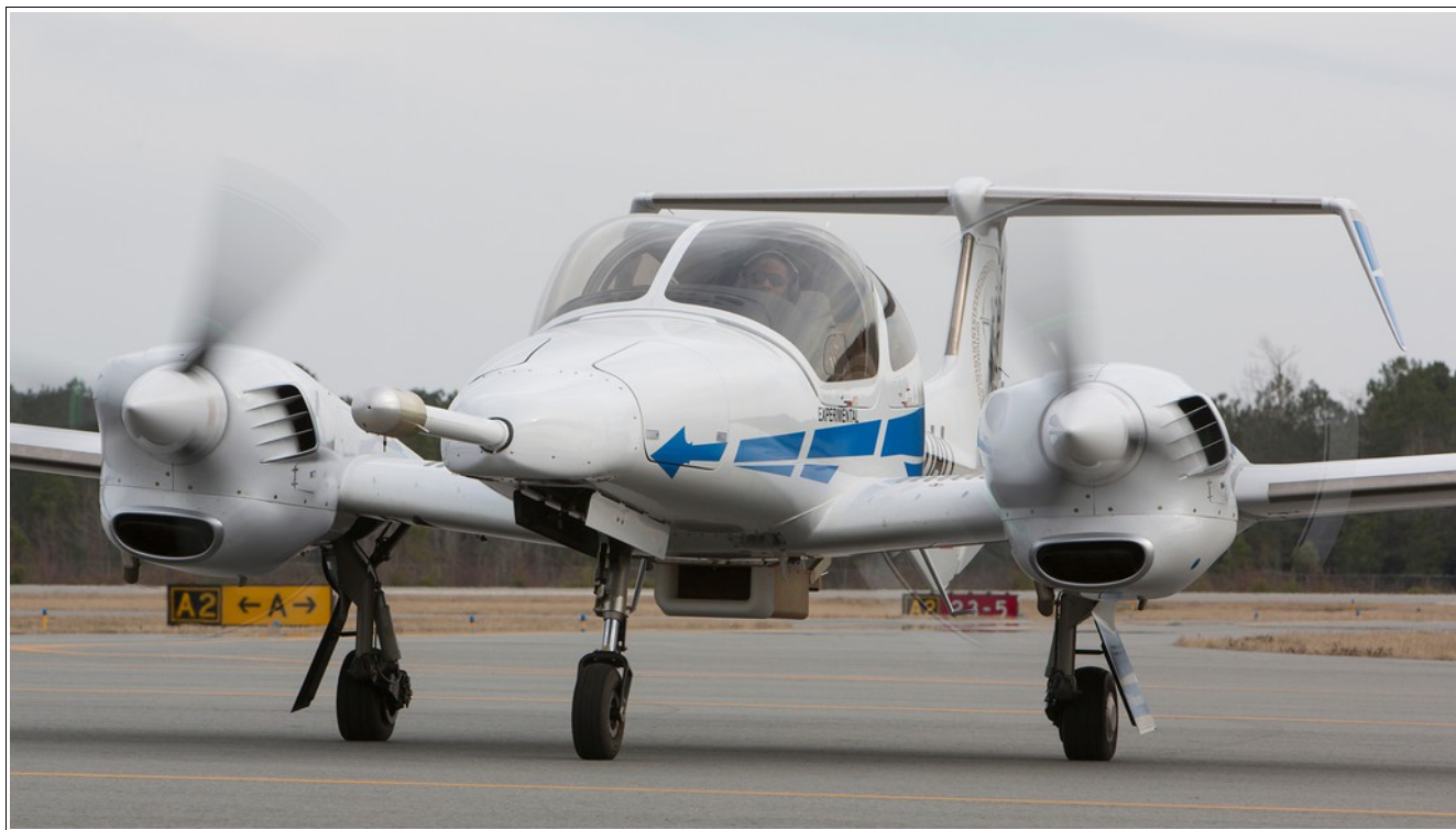
Figure 2. DA-42 with the universal nose and BAT probe.
