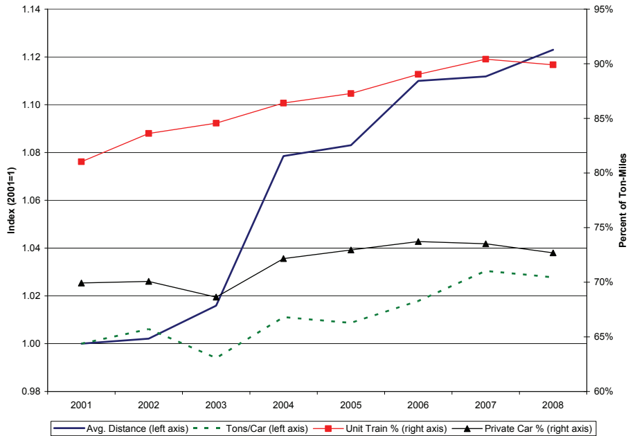
FIGURE 6-3 SELECTED COAL SHIPMENT CHARACTERISTICS INDEXES FOR AVERAGE DISTANCE AND TONS/CAR (LEFT AXIS) PERCENTAGES FOR UNIT TRAINS AND PRIVATE CAR OWNERSHIP (RIGHT AXIS) 2001-2008 CARLOAD WAYBILL SAMPLES
