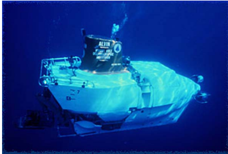
Figure 1-8. Human Occupied Vehicle
