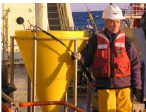
Figure 1-13. Moored Sediment Trap
