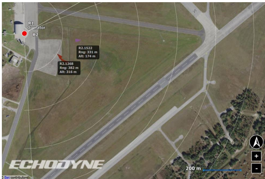
Figure 13: Echodyne software detecting the BST S2 (left target) and Meteodrone SSE (right target). Image taken at 20:30 UTC 5 March 2019.
