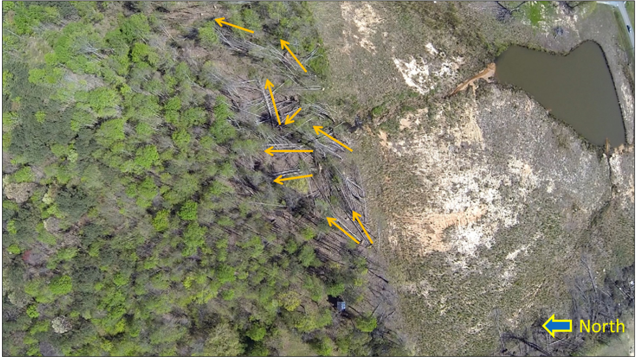
Figure 13: Damage near the middle of the Priceville tornado track on 5 April 2016 from Flight 3. Orange arrows indicate direction trees fell. North arrow indicated in bottom right.
