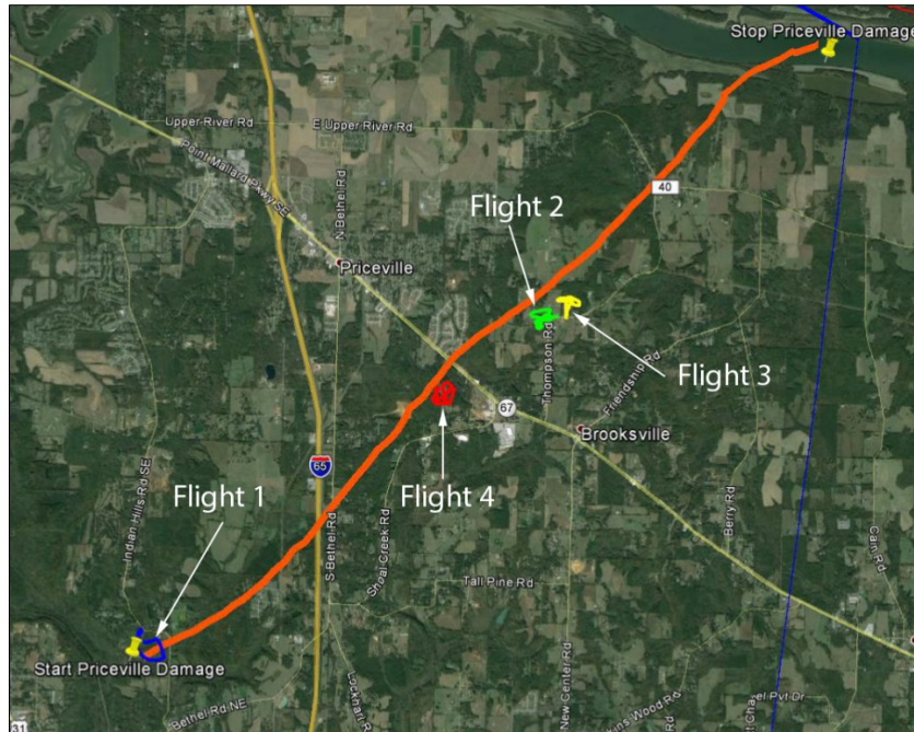
Figure 9: EF-2 tornado damage path (thick orange line) near Priceville on 31 March 2016 and sUAS flights on 5 April 2016. Flights 1, 2, 3, and 4 correspond with blue, green, yellow, and red lines, respectively.
