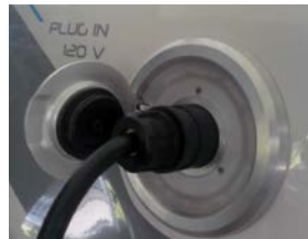
Figure 6-4. Level 1 plug-in hybrid electric vehicle charging port.
