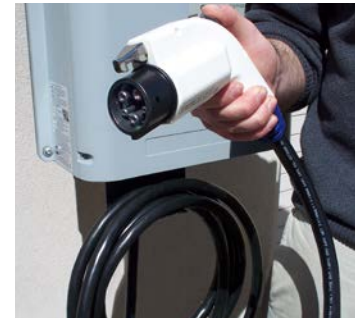
Figure 6-6. EVSE Level 2 charging equipment with a SAE 1772J connector.
