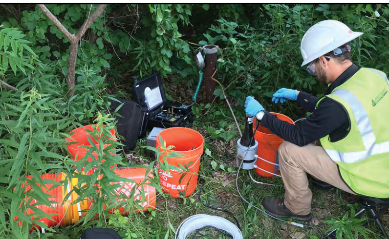
A worker samples groundwater using ‘low-flow’ sampling protocols.
