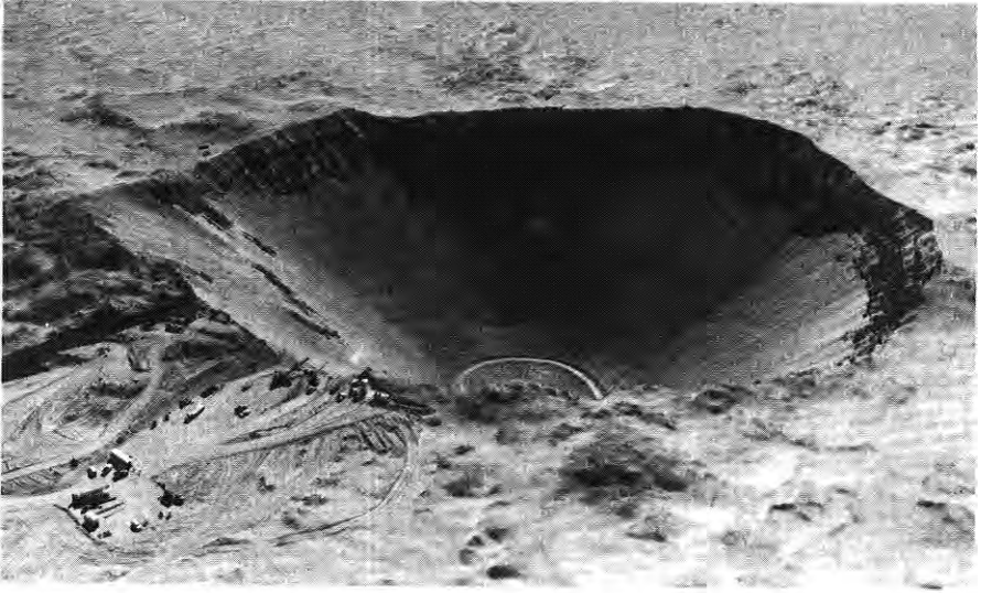
Figure 6.10. SEDAN event; crater formed by a 100-kiloton explosion in alluvial soil at the optimum depth of burst (635 feet) for cratering. The crater radius is 611 feet, the depth 323 feet, and the volume 179 million cubic feet.
