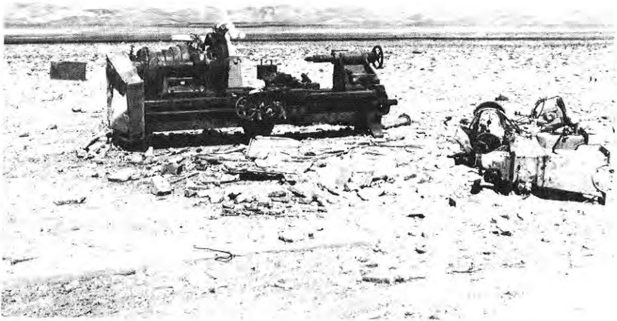
Figure 5.129a. Machine tools after a nuclear explosion (10 psi peak overpressure).
