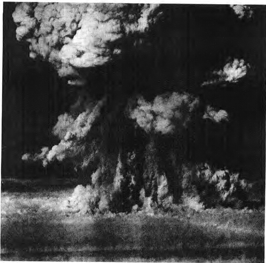
Figure 2.18b. Formation of dirt cloud in surface burst.
