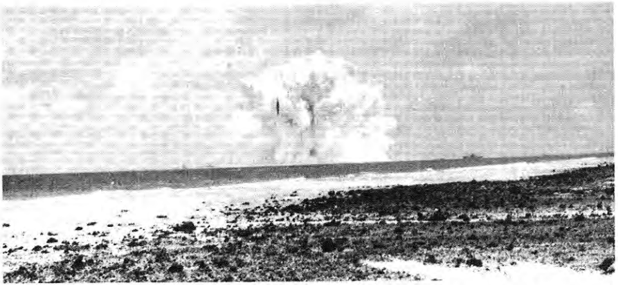
Figure 2.84b. Plume observed 11.7 seconds after explosion in deep water.
