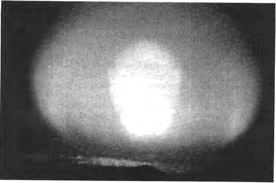
Figure 2.56. Fireball and red luminous spherical wave formed after the TEAK high-altitude shot. (The photograph was taken from Hawaii, 780 miles from the explosion.)
