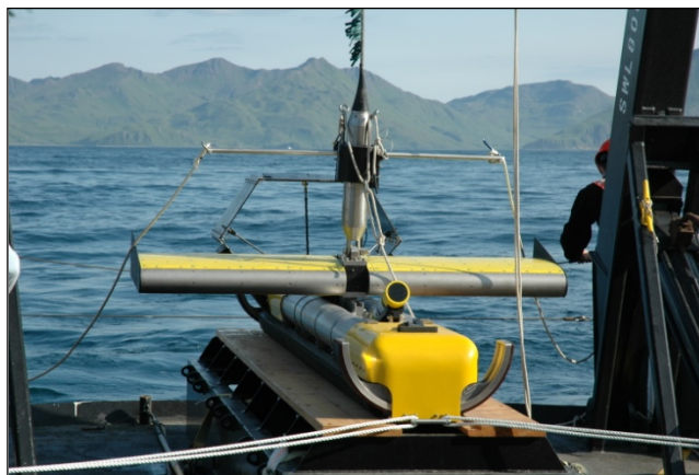
Figure 2: Long-range side scan sonar system for fisheries research.
