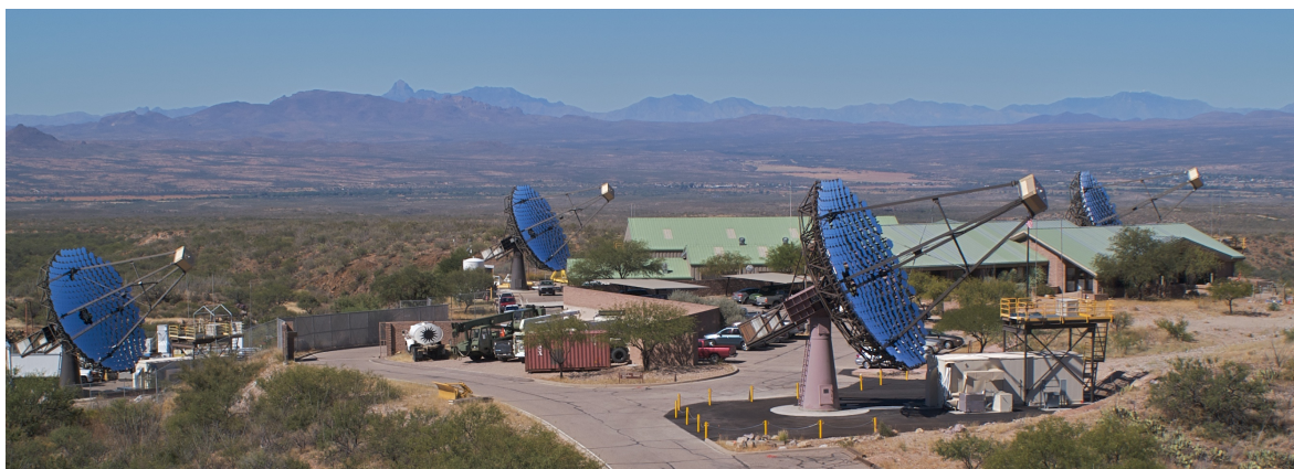
FIGURE 7.10 ACTA would be, like the pictured VERITAS (Very Energetic Radiation Imaging Telescope Array System), an array of Cerenkov telescopes used to detect very high energy (TeV) gamma rays emanating from astrophysical sources. The proposed ACTA telescope would be a larger-scale international version of this facility and similar ones located in Namibia and the Canary Islands that would increase the sensitivity by roughly an order of magnitude. Image courtesy of Steve Criswell, SAO.
