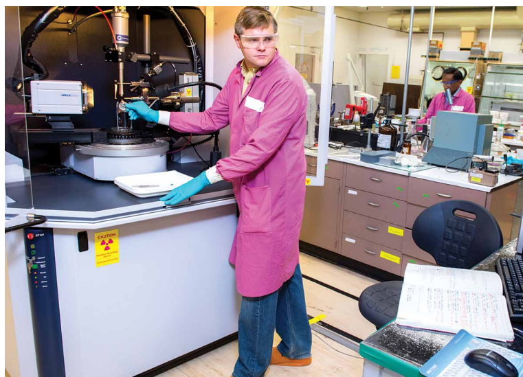
Revealing Molecular Structures of Actinides. Richard Wilson at Argonne National Laboratory (ANL) prepares a single-crystal x-ray diffraction measurement of an inorganic actinide complex. Such measurements reveal the molecular structures of these elements, knowledge critical to understanding their physical and electronic properties. [Image courtesy ANL]
