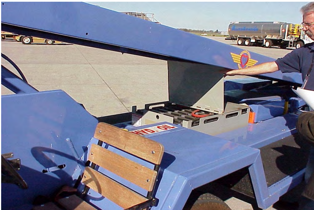
Rick Waugh, Southwest Airlines' Western Region Manager, Ground Support, explains operation of a new SWA electric belt loader to Mustapha Janneh of International Group Technologies and ILEAV consultant to SMF. Below, Rick shows battery location.
