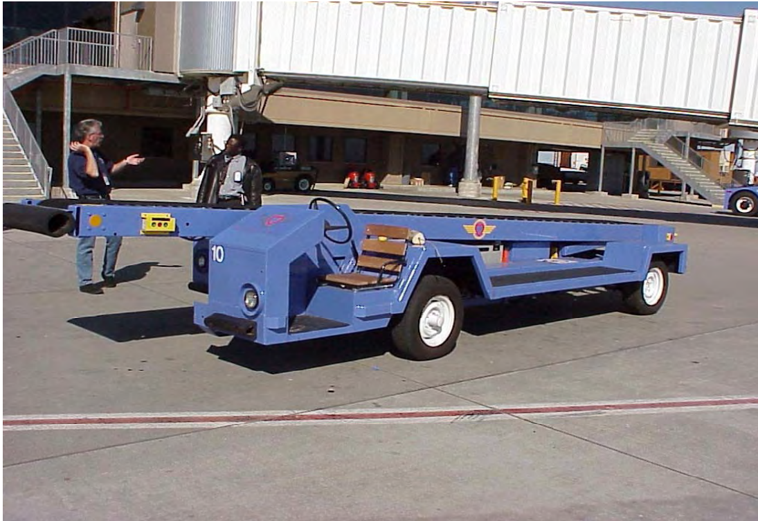
Rick Waugh, Southwest Airlines' Western Region Manager, Ground Support, explains operation of a new SWA electric belt loader to Mustapha Janneh of International Group Technologies and ILEAV consultant to SMF. Below, Rick shows battery location.
