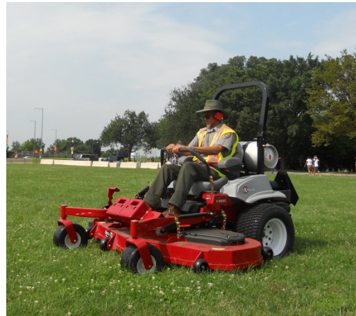
A National Park Service employee operates a propane-powered mower at the National Mall in Washington, D.C. Photo from Julie Sutor, NREL 26748.
