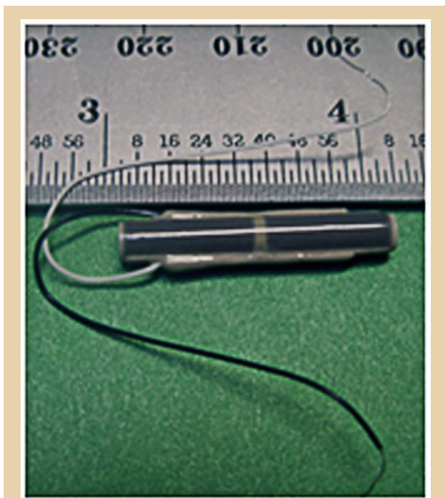
Figure 2.7-1. Electrostrictive adjuster manufactured by Xinetics. When voltage is applied to the device, the length changes. The change in length is stable when the voltage is removed.
