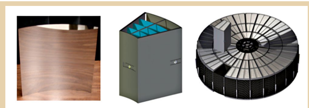
Figure 2.3–1. These images illustrate the main steps in building a hierarchical X-ray telescope. Left: Fabricate large numbers of thin mirror segments. Middle: Align and bond numerous (typically on the order of one hundred) mirror pairs into a mirror module. Right: Co-align and integrate many (tens to hundreds) modules into a mirror assembly.
