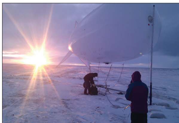
Fig. 9. Tethersonde Test Flight. Tethersondes, like this one, are used to collect atmospheric measurements at the Atmospheric Radiation Measurement (ARM) User Facility’s mobile observatory at Oliktok Point, Alaska. [Courtesy ARM User Facility]
