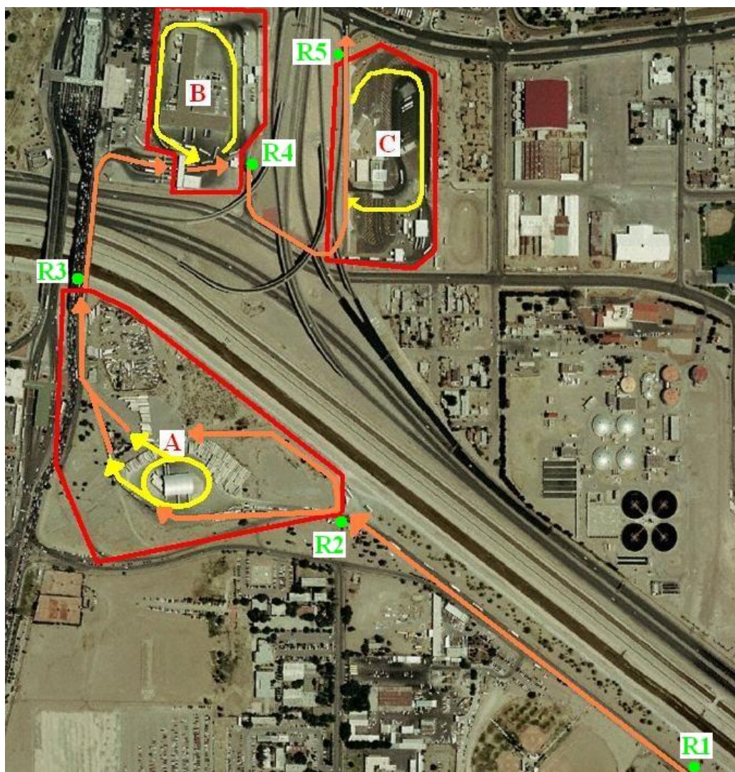
Figure 15. Map. BOTA showing Federal and State inspection facilities and initial RFID reader locations.
