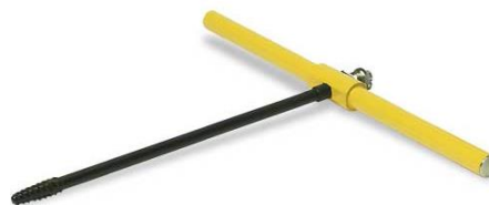
Figure 2-11. Increment corer used to collect hardwood tissue samples.
