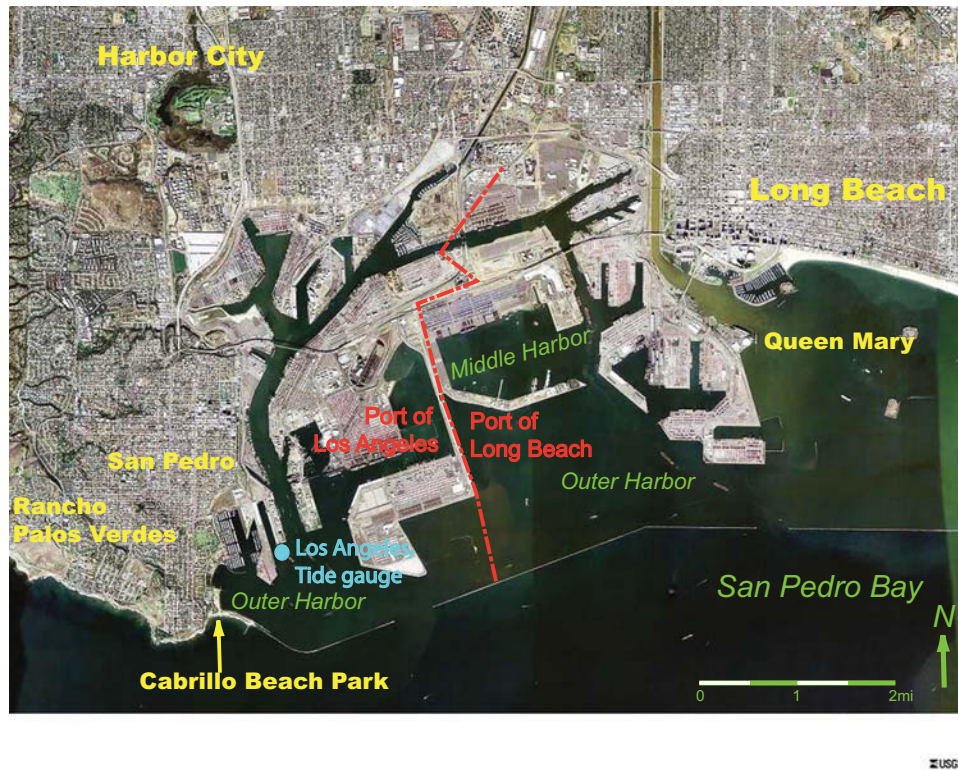
Figure 1.1: Satellite image of the ports of Los Angeles and Long Beach (TerraServer-USA and USGS). The red dotted line demarks the border that separates the two ports. Model validation is based on the Los Angeles tide gauge located at Berth 60, as shown and marked in blue. The low elevations surrounding the ports of Los Angeles and Long Beach make the region vulnerable during a tsunami event. Residents of the densely populated cities of San Pedro, Harbor City, Long Beach, and Rancho Palos Verdes, along with the many tourists that visit attractions, including Cabrillo Beach Park, the Queen Mary, and the Aquarium of the Pacific, are at risk from tsunami impact.
