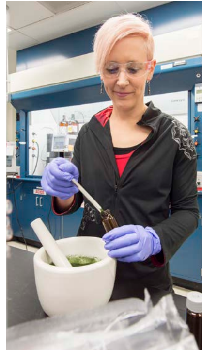
An NREL scientist homogenizing biomass in the Compositional Analysis Lab in the Field Test Laboratory Building at NREL. Photo by Dennis Schroeder, NREL.
