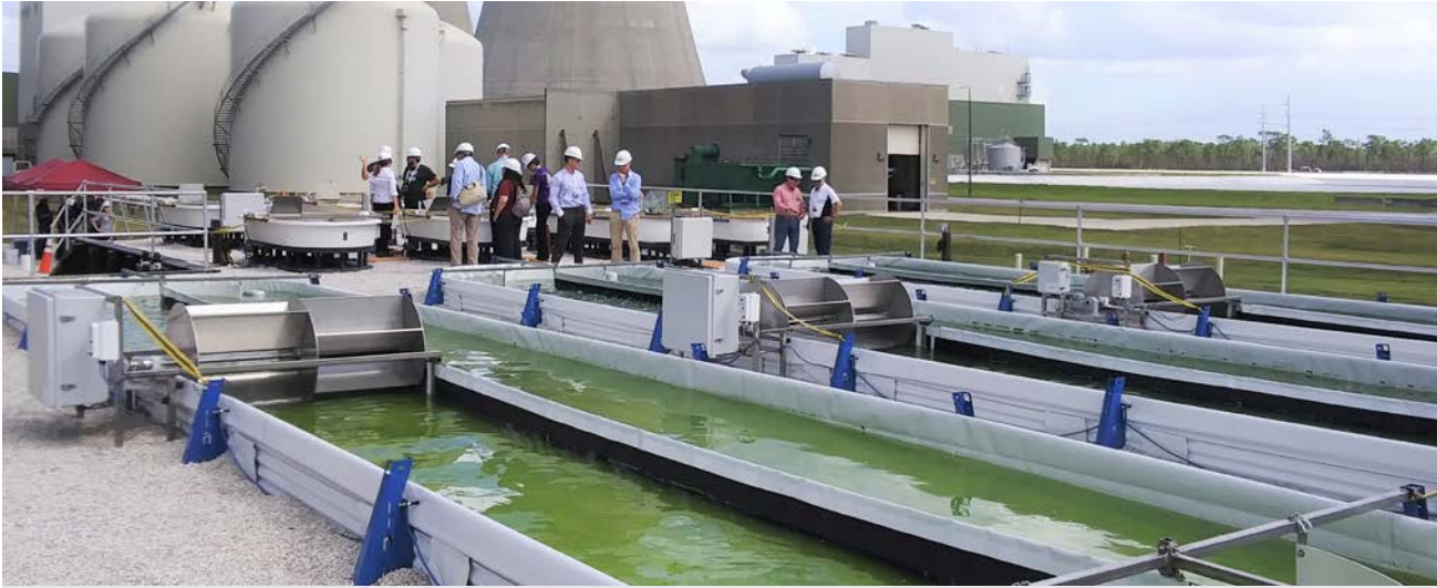
Demonstration testing of direct flue gas injection into a filamentous algae open system operated by the Orlando Utilities Commission at the Stanton Energy Center and MicroBio Engineering Inc. Photo by MicroBio Engineering Inc.
