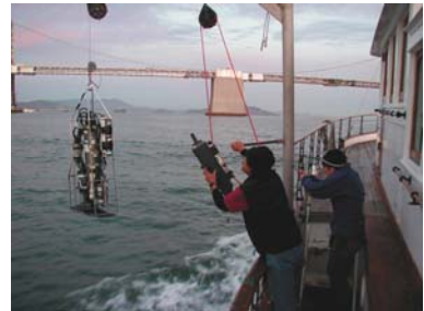
Hydrologists collect water samples for analysis of long-term trends in nutrients, dissolved oxygen, chlorophyll a and other constituents in San Francisco Bay.
