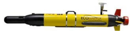
Automated underwater vehicles (AUVs) are used in the bay of Green Bay and the Milwaukee harbor environments, and produce continuous high-resolution data for chlorophyll a , temperature, conductivity, dissolved oxygen, pH, turbidity, and blue-green algae. (Note: AUVs, such as the YSI Ecomapper shown above, are available from a variety of manufacturers.)
