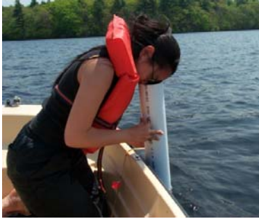
A volunteer lake monitor views a Secchi disk through a view tube to monitor water clarity (or transparency,) an important indicator of water quality. (Photograph by Elizabeth Herron)
