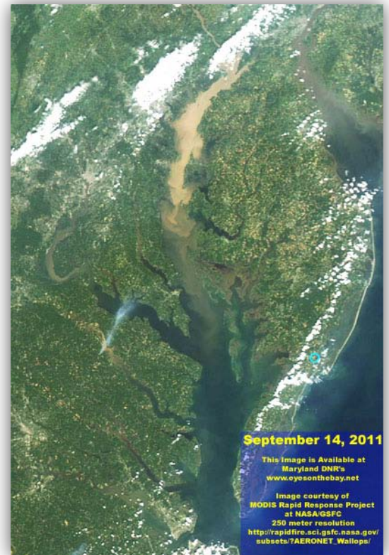
Figure 2. Sediment plume associated with storm runoff moving down the Chesapeake Bay days after Tropical Depression Lee passed through (Chesapeake MODIS Satellite Imagery and Data). Source: http://mddnr.chesapeakebay.net/eyesonthebay/satellite_result.cfm#picview
