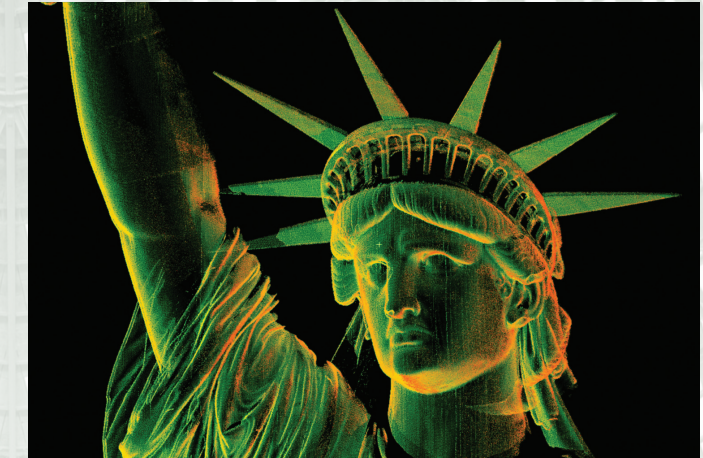
Statue of Liberty, New York, New York, HAER office. Point cloud data is produced from a high-definition laser scanner.
