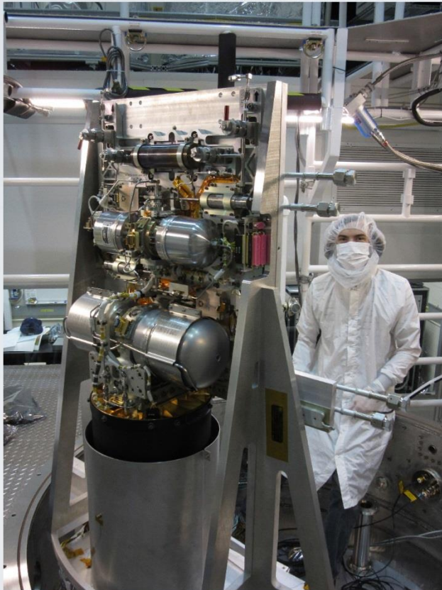
Compressor Assembly and deployable refrigerant line
