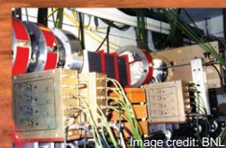
Heavy Ion Testing of Inflatable Shield Prototype
