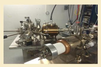
Figure 1: Over 20 years of R&D have dramatically increased the performance of polarized electron sources. Foreground: early-generation source. Back: recent load-lock, ultra-high vacuum source using super-lattice GaAs/GaAsP photocathodes. Such sources can deliver a record 4 mA, 90% polarized electron current.
