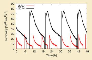
Figure 2: A breakthrough in stochastic beam cooling was able to overcome the internal heating process of the high-energy heavy-ion beams of the Brookhaven RHIC and reduce the beam width up to fivefold. With the brighter beams, the collision frequency or luminosity was vastly increased.
