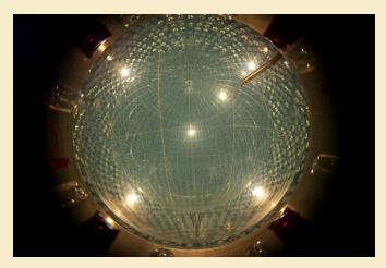
The Borexino detector in the Gran Sasso underground laboratory in Italy.
