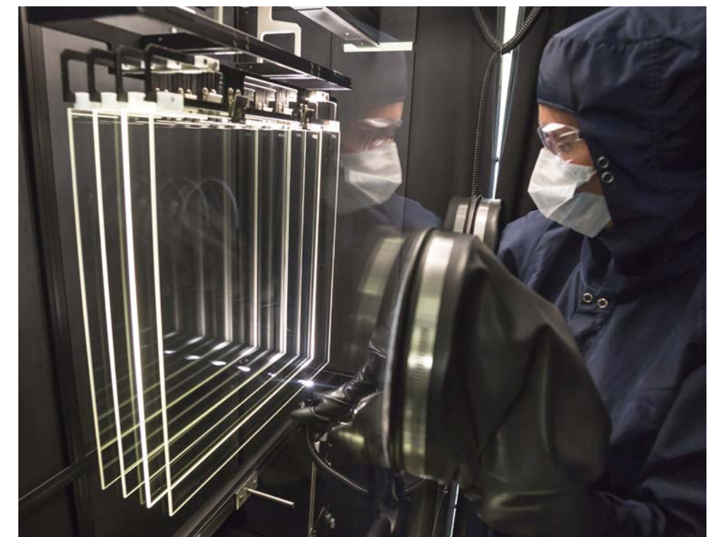
At the National Ignition Facility, a low-cost disposable debris shield (several are shown here) protects the final optics from debris and contamination. However, the disposable shield is susceptible to damage, which, in turn, can cause glass shards and particulates to be introduced into the optical field.
