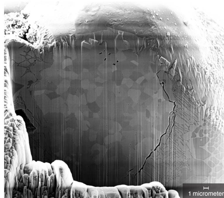
Staff and students at the Naval Postgraduate School have characterized burn residue to help the Livermore team better understand the thermite reaction mechanism. A magnified sample is shown.
