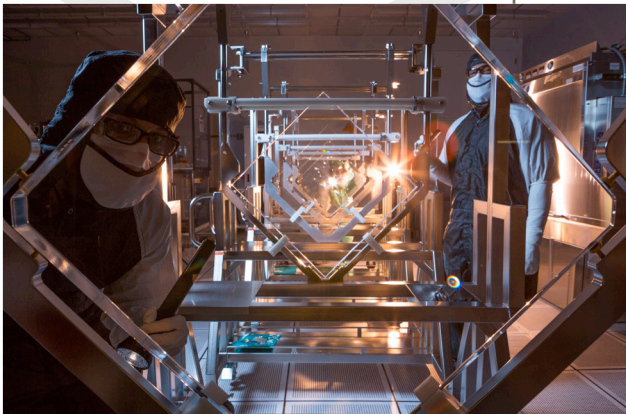
Weged focus lenses and grating debris shields for the National Ignition Facility are processed in LLNL's Optics Processing Facility.
