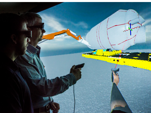
Above: Laboratory demonstration of SRNL Virtual Reality training program designed to improve workers’ abilities to safely and efficiently disassemble the massive converters and associated process components in the Portsmouth Gaseous Diffusion Plant; Below 3D visualization to determine optimal locations for deployment of GrayQb™ device clusters in Hanford Plutonium Reclamation Facility canyon
