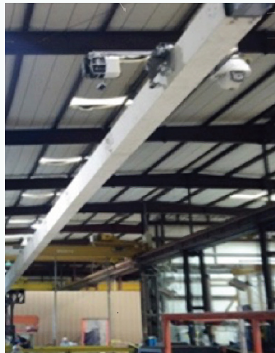
Camera boom designed by SRNL (pictured in laboratory, left, and in underground room containing breached drum at WIPP, above) investigated the cause of WIPP radioactive release.
