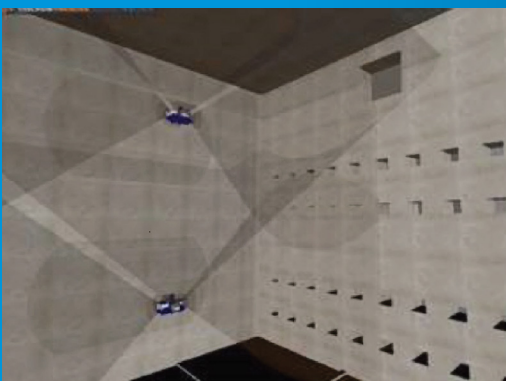
Above: Laboratory demonstration of SRNL Virtual Reality training program designed to improve workers’ abilities to safely and efficiently disassemble the massive converters and associated process components in the Portsmouth Gaseous Diffusion Plant; Below 3D visualization to determine optimal locations for deployment of GrayQb™ device clusters in Hanford Plutonium Reclamation Facility canyon
