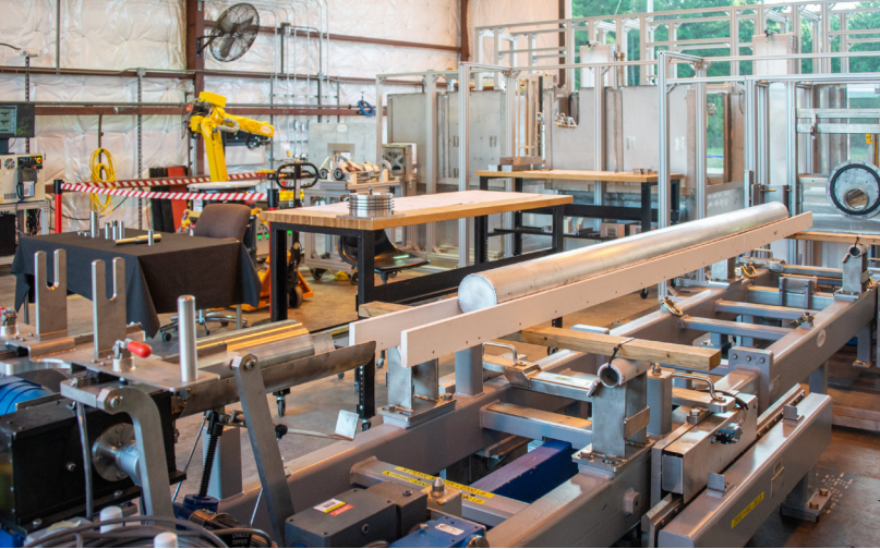
Top Left: Equipment for the plutonium-244 recovery campaign in the SRNL mock-up facility; Top Right: Commercial robotic arm typically used in a non-radiological environment adapted by SRNL to remotely remove the radioactive material from the shielded workspace and place it in a shielded container for transport.
