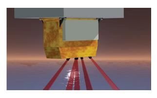
SPEXone polarimeter, planned to be contributed by the Netherlands. It will be excellent for aerosol characterization and address aerosol climate objectives beyond those required of the OCI.
