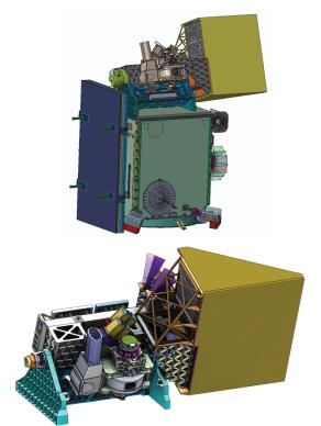
PACE observatory design concept. Ocean Color Instrument (OCI) is at top. Two polarimeters (HARP-2, SPEXone) are located at far right, below the OCI. Folded solar panels are shown at far left.
