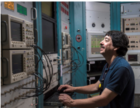
Phil Torrez makes adjustments to the new digital LLRF system at Module 3 of the LANSCE accelerator.
