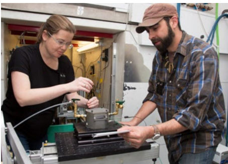
Ann Junghans (left) and Erik Watkins prepare an experiment on Asterix, a polarized neutron beam spectrometer for studies of material surfaces and interfaces.
