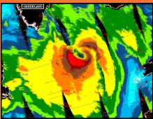
OPC forecasters use a suite of sophisticated tools to assist in marine prediction. In the image above, the scatterometer flying aboard the EUMETSAT METOP satellite measures sea surface roughness, a proxy for ocean surface wind speed and direction. The bright red vectors indicate hurricane force winds; brown storm force; and yellow gale force winds.
