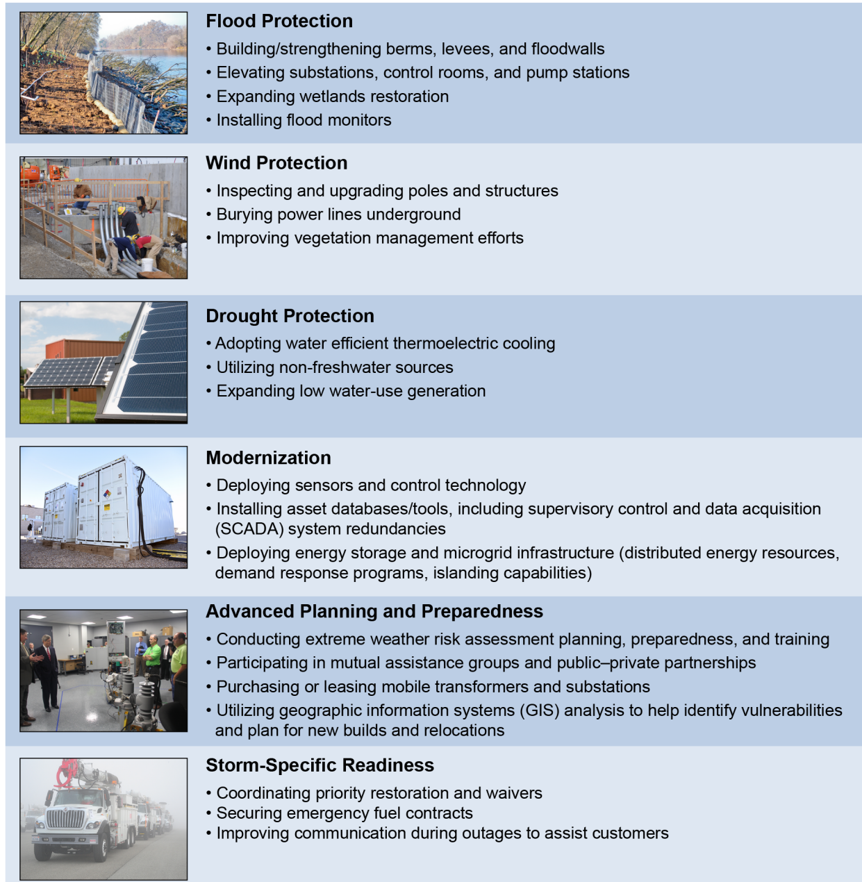
Figure 4.5: Solutions are being deployed in the energy sector to enhance resilience to extreme weather and climate impacts across a spectrum of energy generation technologies, infrastructure, and fuel types. The figure illustrates resilience investment opportunities addressing specific extreme weather threats, as well as broader resilience actions that include grid modernization and advanced planning and preparedness. Photo credits (from top): Todd Plain, U.S. Army Corps of Engineers; Program Executive Office, Assembled Chemical Weapons Alternative; Lance Cheung, USDA; Idaho National Laboratory (CC BY 2.0); Darin Leach, USDA; Master Sgt. Roy Santana, U.S. Air Force.
