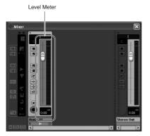
The recording level for Cubase 4 LE can be checked by the level meter of the corresponding channel of the recording enabled track.
