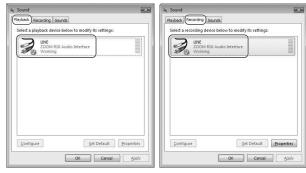
In the "Sound" window, verify that "R16 Audio Interface" is listed under the Play and Record devices and that the device is checked. (To switch between Play and Record, click the tabs at the top of the window.)
