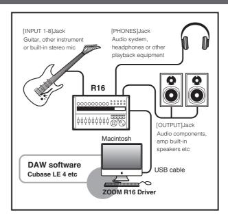
When the connection is operated on the R16, it is recognized by the computer.
